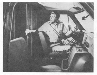
**Sliding partition** between driver's seat and load compartment. Helps protect against shifting load, safeguards cargo because it can be padlocked.
