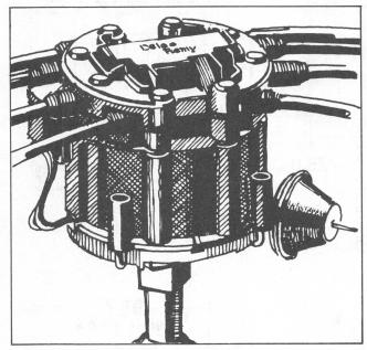
**High Energy Ignition system** • Magnetic pulse generator, electronic control module replace points, condenser and rubbing block • Coil designed for 85% hotter spark than conventional systems.
